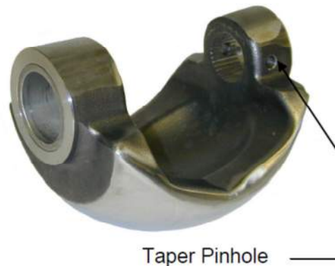
Figure 2. V-Ball showing Groove Pin Hole
